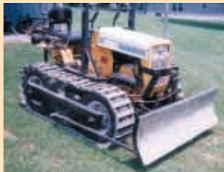
Another one of his tractors is a Cub 122. He fitted it with a dozer blade and tracks.
