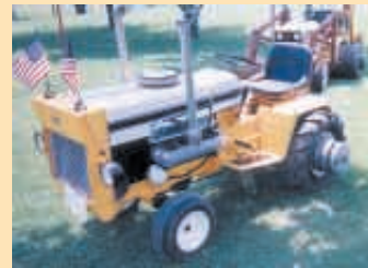
He made this tractor by taking parts from two tractors so he could install a V-8 engine.
