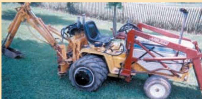
Loren Arledge chopped up and rebuilt a Cub Cadet in order to fit it with a backhoe and loader.
