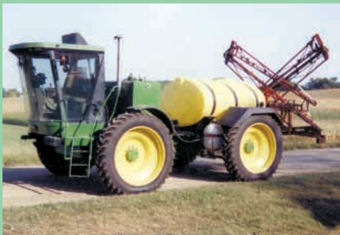
Dennis Cotter built his own articulated, self-propelled sprayer from a 1984 PixAll sweet corn picker.
