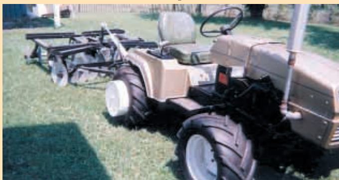
This articulated tractor was also built from two tractors.
