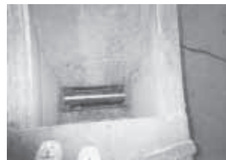
Funnel-shaped hopper at top of cylinder feeds potatoes to knives.
