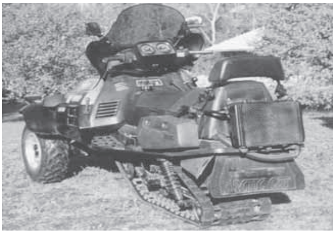
Raymond Maguire combined an Arctic Cat snowmobile, a Bombardier jet-ski, and a Suzuki ATV to make this machine that runs equally well on land, snow or water.
