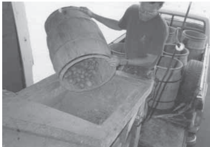
Chopper processes 165 lbs. of potatoes in about a minute, cutting them into 1/2-in. or smaller pieces.
