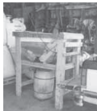
Barrel underneath knives and hopper collects the cut-up potatoes.
