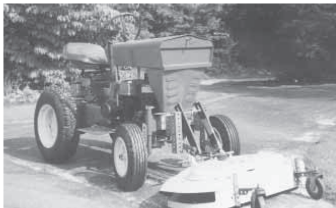
Front-mount mower was made out of a 1967 Mustang riding mower and a 1970’s Ford riding mower, both of which were originally equipped with belly-mount decks.
