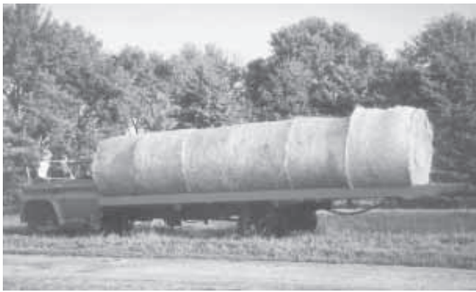
"I can load straw bales on-the-go and have a load in as little as 5 to 7 minutes," says Jerry Jansen, who converted an old 2-ton truck into this self-propelled bale hauler.
