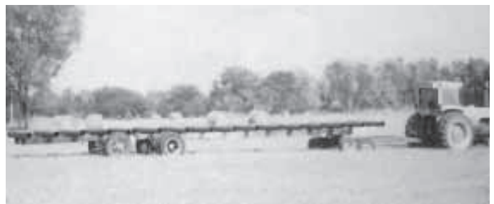
Bill Bower used the frame of an old school bus to make this bale-hauling trailer. He lengthened the frame 22 ft. and made a tandem axle, fifth wheel dolly on front.
