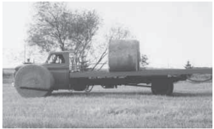
Truck is equipped with a lift arm that mounts direct to truck frame. Jansen can load and carry ten 5-ft. bales or twelve 4-ft. bales at a time.
