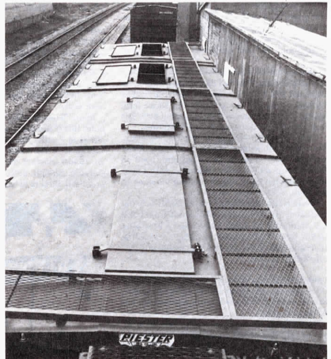
Each coal car top has four 2 by 8 ft. doors for filling the four compartments with grain.
