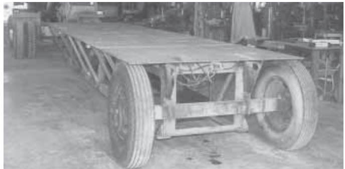
Clair Wilson turned a big slab of 1/2-in. thick steel plate into this giant rolling work bench.
