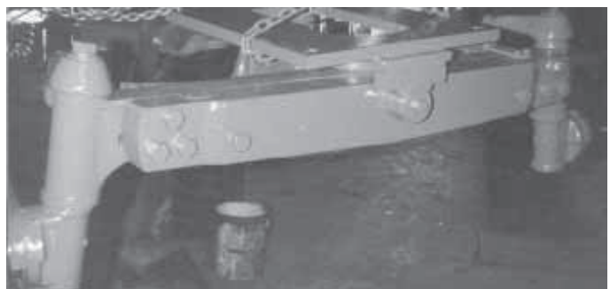
Ed Beem modifies axles to be stronger, wider and to fit other tractors. This John Deere 4640 axle was rebuilt to fit a 4020.
