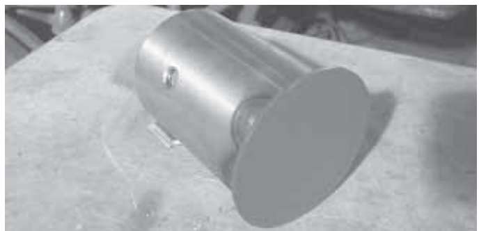
Steel "pipe plug" was adapted to fit the 3 1/4-in. dia. opening left when a tractor's pulley casting was removed.
