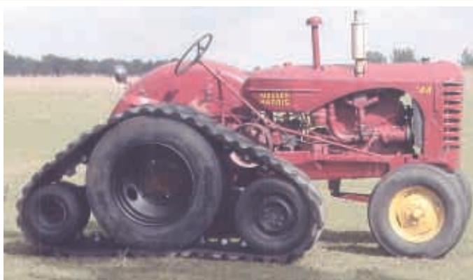
Henry Toews says his new add-on track system is different because the walking beam hangs off the tractor axle, eliminating obstructions outside the wheel.
