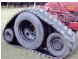
Prototype uses tractor tires to form an endless track.
