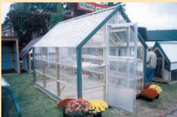
Portable greenhouse, like most of Samuel's buildings, mounts on 4 by 6 wood skids. A pair of hooks at each end makes building easy to move around.
