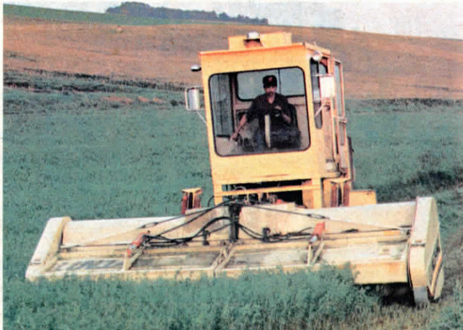
In addition to cutting hay and grass, the auger mower also "works great" to cut and windrow corn stalks for baling.
