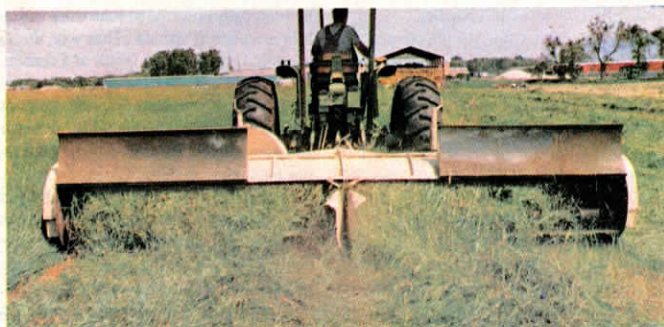
Short stub augers behind cutter auger fluff hay as they feed it out into side-by-side windrows.
