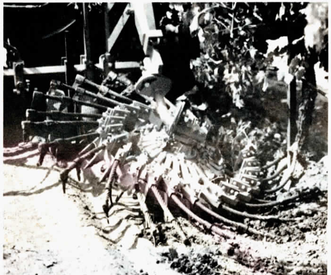
Metal teeth clamped to lengths of 7/8-in. dia. steel cable cut and rake out weeds.
