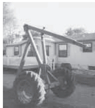
Home-built crane was built out of the front drive axle off a Deere 45 self-propelled combine.
