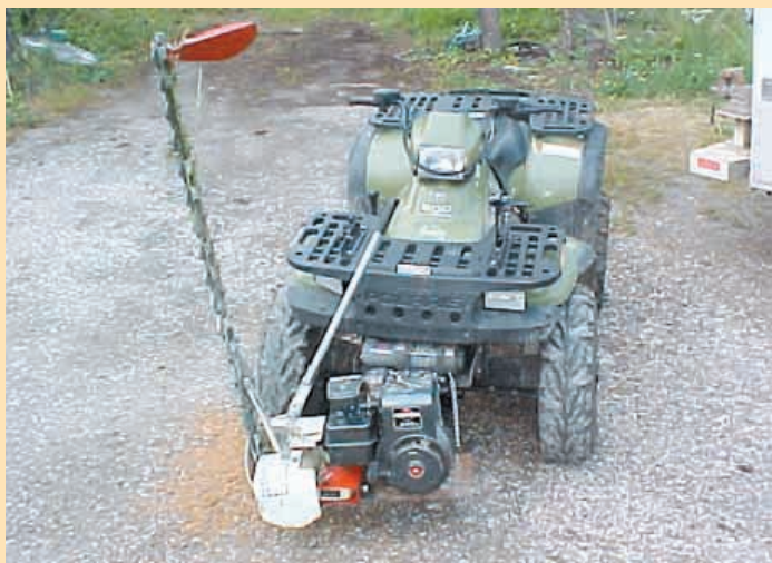
He removed the pto hardware so he could drive it with an engine. A winch on front is used to lift sicklebar up.
