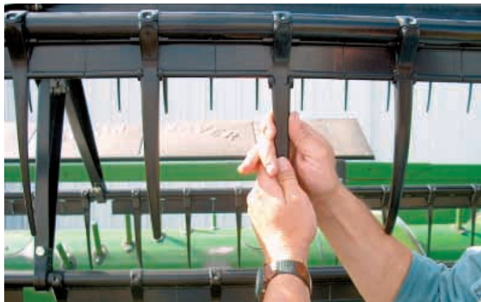
Quick Fingers slip over broken reel tines and simply snap into place.
