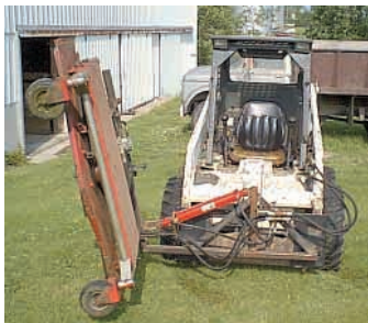
Unit hinges up and down on two pins and quick couples to skid steer's auxiliary hydraulics.
