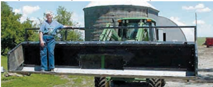
Loader-mounted scaffold is built from an old 14-ft. combine header. Bucket-mounted bracket is used to hold scaffold on Schweppe's Deere 7320 tractor.
