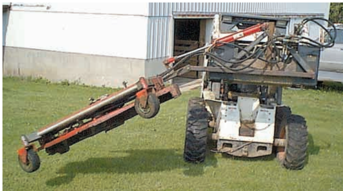
"It works great for cutting along fences and roadsides," says James Boyd about the 5-ft. mower he built out of an old commercial Gravely walk-behind mower.
