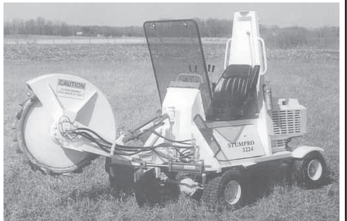
StumPro has a huge circular saw on front. After reducing stump to chips, you can lift saw blade out of the way and use machine's front blade to push dirt and chips back into hole.
