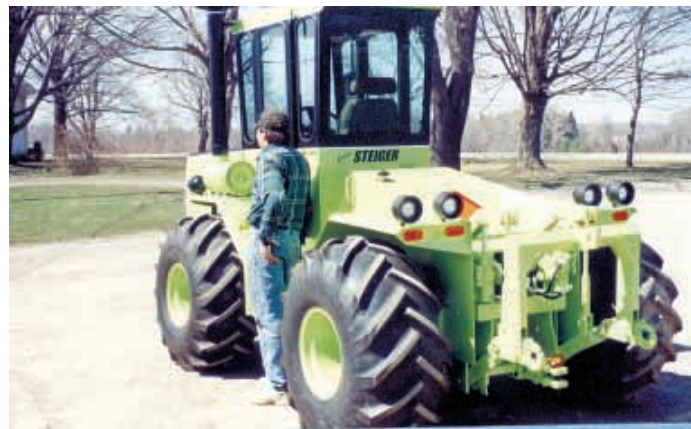
Using mostly scrap material, David Agle built his own half-scale working model of a Steiger tractor. Power is supplied by a 4-cyl. gas engine.
