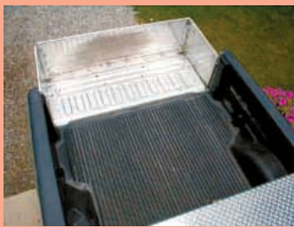
Pickup "bed extender" is made of aluminum panels that add 24 in. to length of truck box.
