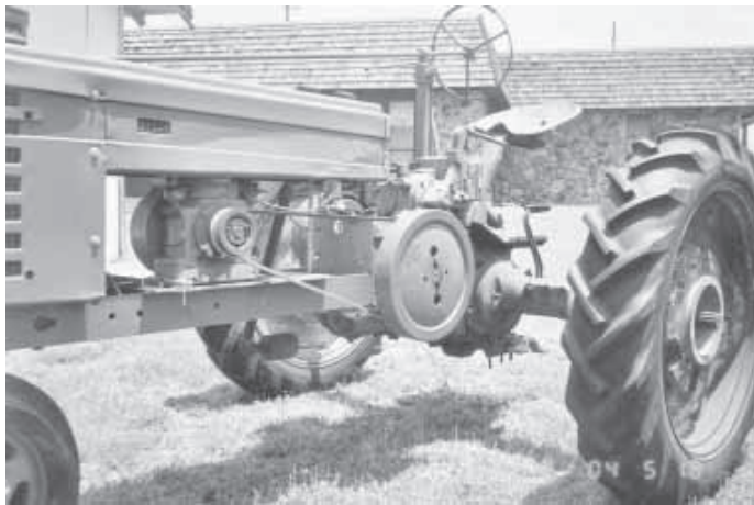
Powered by an 8 hp Briggs & Stratton engine, Bobby McCowen’s Deere H tractor rolls along at a top speed of 8 mph.
