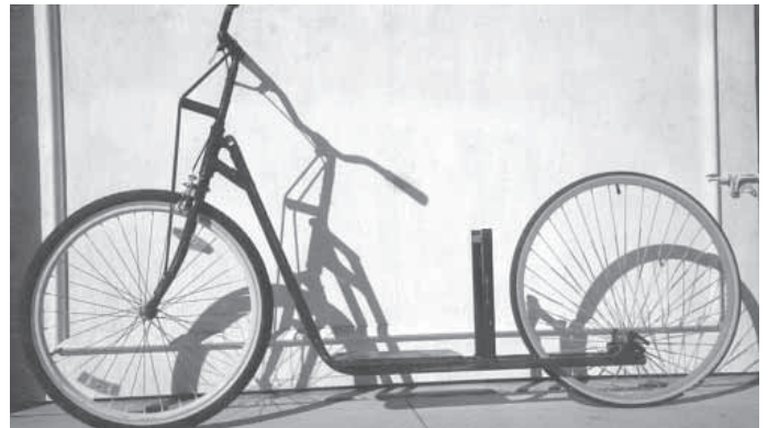
Scooter’s rear wheel has an off center axle with a series of uneven spokes welded to it. Axle is connected to a metal frame that rider stands on.
