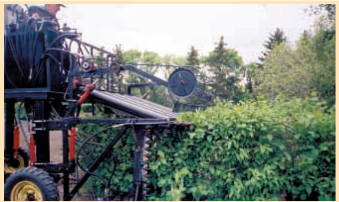
Machine trims hedges from 6 1/2 to 3 1/2 ft. high. Draper canvas behind top sicklebar carries trimmings off to side.
