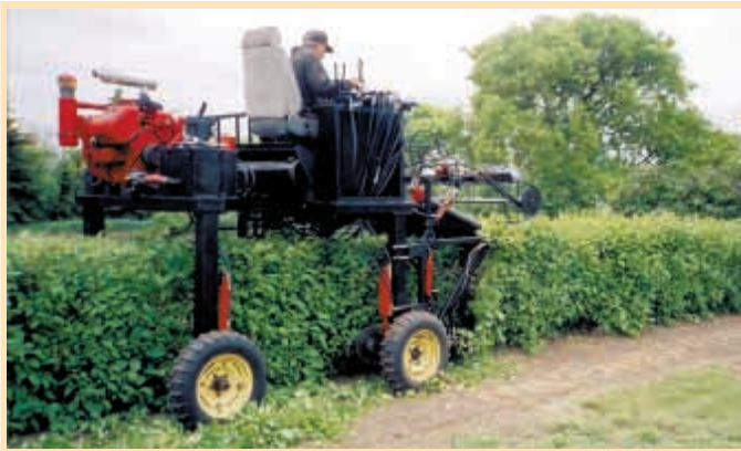
Hydraulic-powered hedge trimmer uses three sicklebars to cut hedges on all sides of hedge at once.
