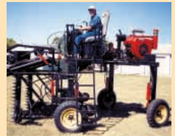
Rigs four legs are each equipped with a hydraulic cylinder, allowing entire machine to be raised or lowered up to 8 in.
