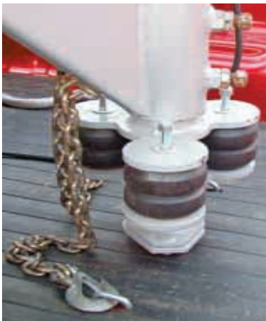
Three Timbren rubber springs absorb shock. "Having an improved ride is nice, but reducing the jerk between the truck and trailer really impressed me," says Mr. Truck.
