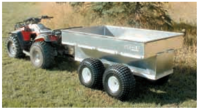
Largest model ATV trailer, made of steel or aluminum is 6-ft. long and 5 ft. wide and carries up to 2,000 lbs.
