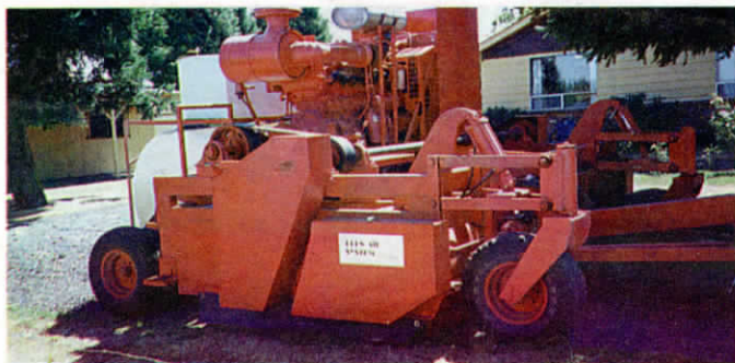
The machine makes a vacuum that sucks residue into the hammermill which then "totally pulverizes" all crop material and deposits it back on the ground.
