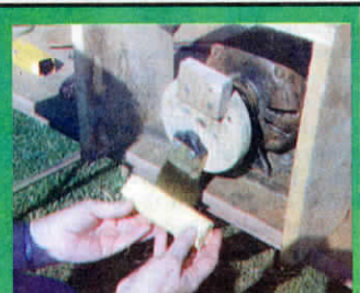
De-silker uses a 1/4 hp electric motor to "power" a paint brush.
