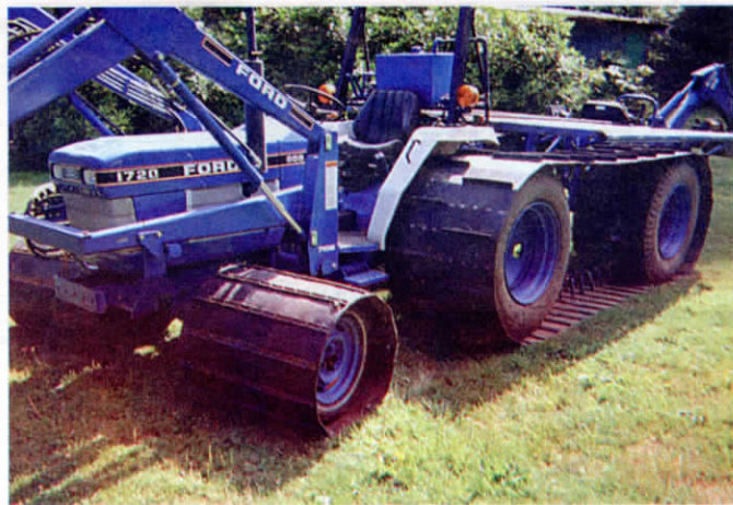
New track system makes use of an add-on axle that mounts behind tractor's original rear axle. Each track is held in place by a row of steel spring guides.
