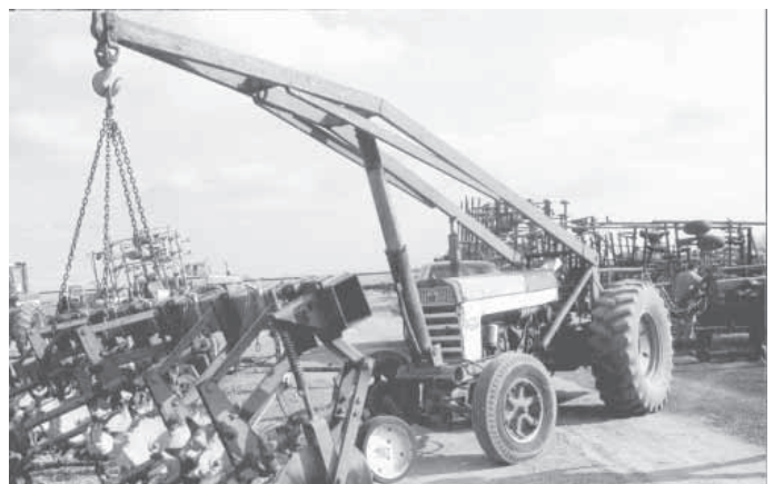
Lift can hoist a load up to 6,000 lbs., raising it as high as 18 ft. in the air.
