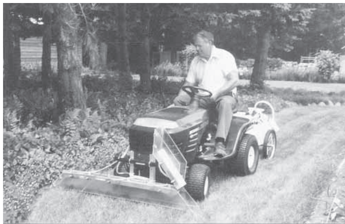
A bank of 4 valves controls the center section and each wing. Plastic guard prevents drifting and holds flowers out of herbicide's path. Left wing in photo is up.
