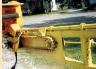
Chain saw attaches to roller chain that's moved back and forth by rod that runs back along top of framework.
