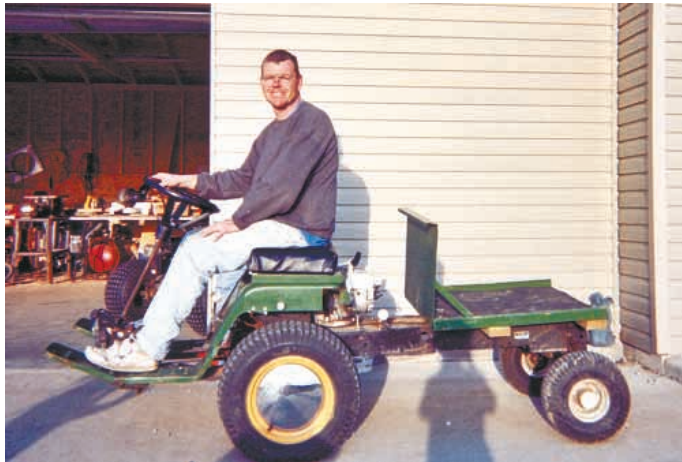
Busse mounted floorboards and pedals onto an extension of frame ahead of drive wheels.
