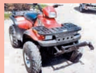
Telescoping hitch attaches to a metal bracket bolted to front of ATV. It folds out of the way when not in use.
