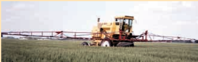
Penner removed feederhouse and mounted a 90-ft. boom on front. He also removed the cylinder, concaves and straw walkers to make room for a home-made spray tank. Thresher clutch powers sprayer pump.
