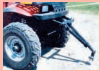
Telescoping hitch attaches to a metal bracket bolted to front of ATV. It folds out of the way when not in use.
