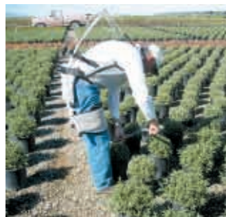
Fiberglass rods attach to chest harness and leg straps, providing lift that supports back.
