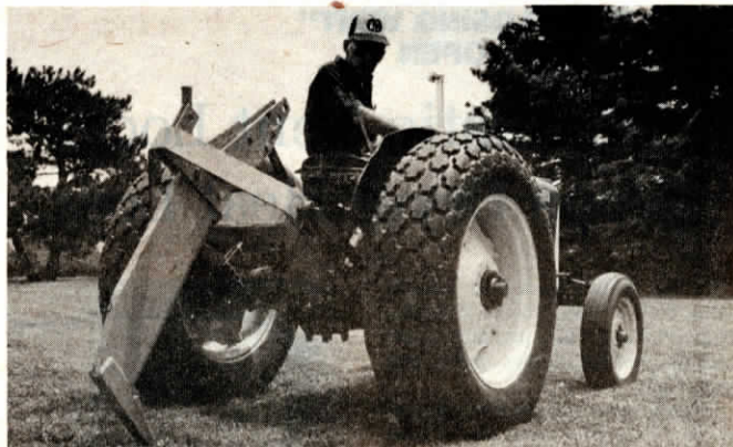
Plow digs 20-in. deep to cut through lateral "sucker" roots of hedge trees. A 50-hp. tractor can clean up 1/2 mile per hour.
