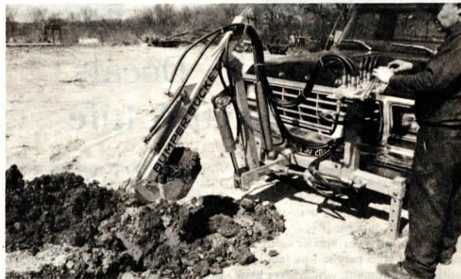
Backhoe digs as deep as 55-in. and has an 88-in. reach.
