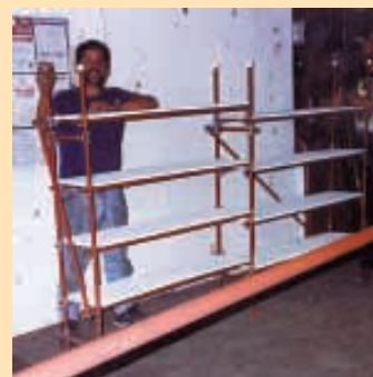
Many different sizes of clamps are available. The smallest connects 1/4-in. pipe to 3/8-in. pipe, and the largest connects 4-in. to 8-in. pipe.
