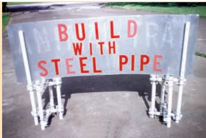
Many different sizes of clamps are available. The smallest connects 1/4-in. pipe to 3/8-in. pipe, and the largest connects 4-in. to 8-in. pipe.
