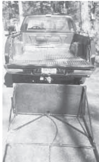
"Truck sled" fits inside the bed on Tuggle's 3/4-ton pickup. A chain runs from front of sled to back of truck. To remove load, Tuggle lowers tailgate and hooks chain up to a tree or building, then drives pickup forward out from under the load.
