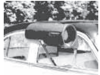
Hot outdoor air is channeled through window-mounted car "cooler" and cooled by evaporating water in the unit.
