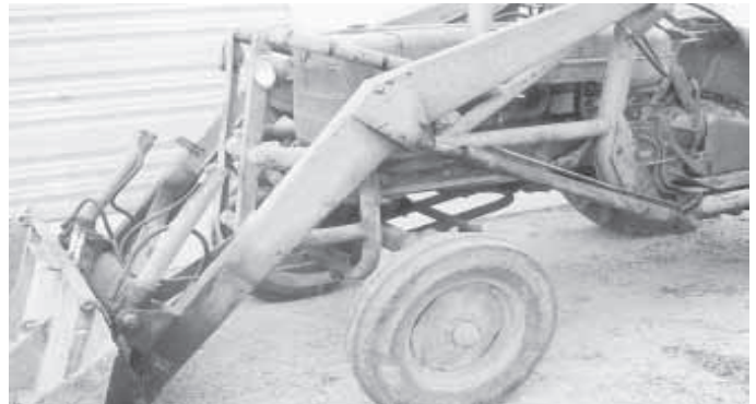
James Marley modified an old Ford front-end loader to fit his 1945 Allis Chalmers D-14 tractor, which had no hydraulics. Loader frame doubles as oil reservoir.
