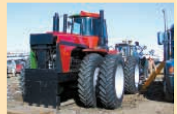
Giant hinge plate on front of tractor holds tractor in place.
