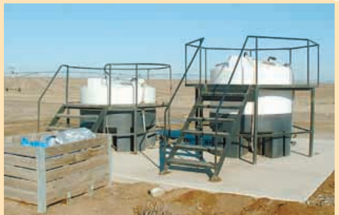
Compost tea is brewed in 1,000-gal. batches using giant “tea bags” filled with worm castings, cow manure, kelp and molasses. The tea is used as a soil conditioner.
