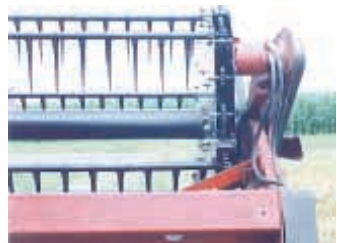
New reel drive system changes angle of pickup fingers and how they handle crop.
