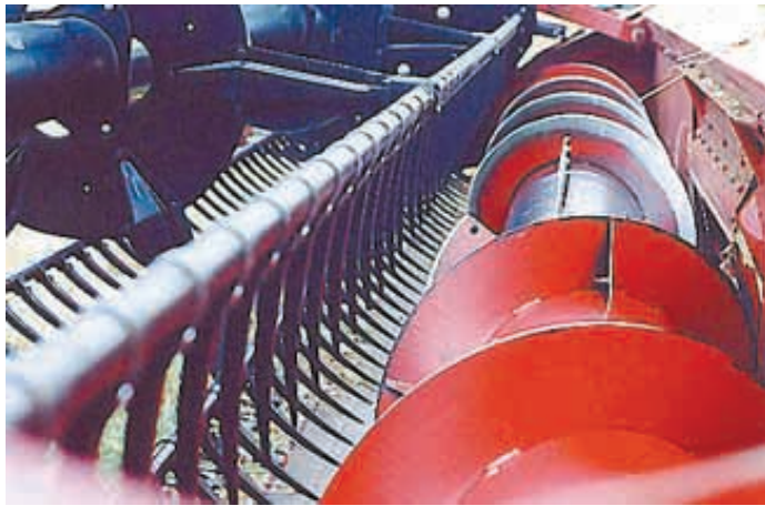
Fingers on modified reel follow contour of auger as they convey crop into header.
