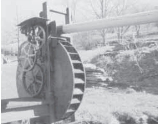
To make the water wheel, he cut off both ends of a large oil tank to make the sides and then welded in buckets from an old grain elevator.
