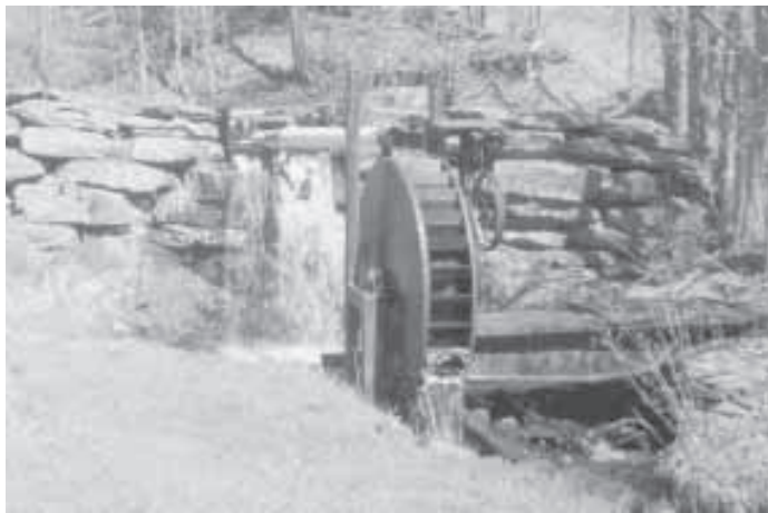
Finch hauled in big rocks to dam up a stream that runs through his property. Water flows through a large pipe to water wheel.
