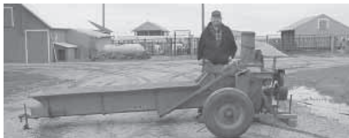
Schweppe converted this silo blower - equipped with an 11-ft. conveyor - into a “feed thrower” by removing blower and moving wheels and axle under center of conveyor.
