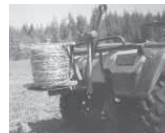
Dave Elmquist used sq. steel tubing and 1-in. dia. pipe to make a removable barbed wire roller for his Honda 4-wheeler. Hooks catch on ATV rack (right).
