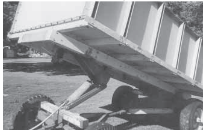
Wagon is equipped with a hoist cylinder off another wagon. It dumps out the back.
