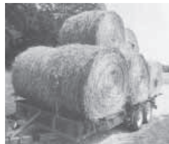
Trailer can haul up to eight 4 by 5 round bales at a time.
