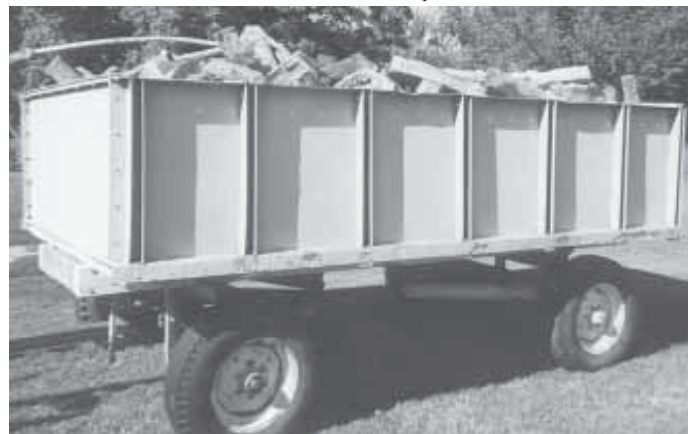
Lyle Torstenson made this 8 by 12-ft., 8-ton wagon using galvanized sheet metal off an old continuous flow grain dryer and the steering axles off a pair of Deere 95 combines.
