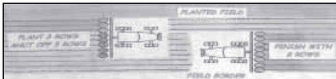
If you use an 8-row planter and have 11 rows left to plant in the field, you can shut off 5 row units on the next to last pass and then finish planting field using a full eight rows.
