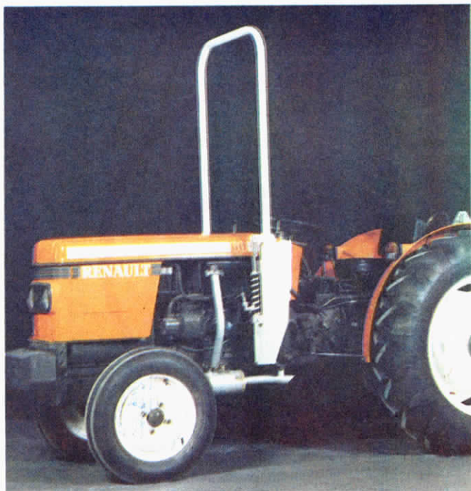
Buisard's rollbar lowers hydraulically for close-in maneuverability and storage.
