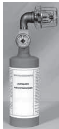
"Watchguard" is activated by heat at 165 degrees. At that point it automatically discharges a non-toxic dry chemical out of a sprinkler head.
