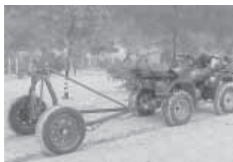
Herb Linderman used 2-in. sq. tubing to make the frame and arch for his 2-wheeled skidder.
