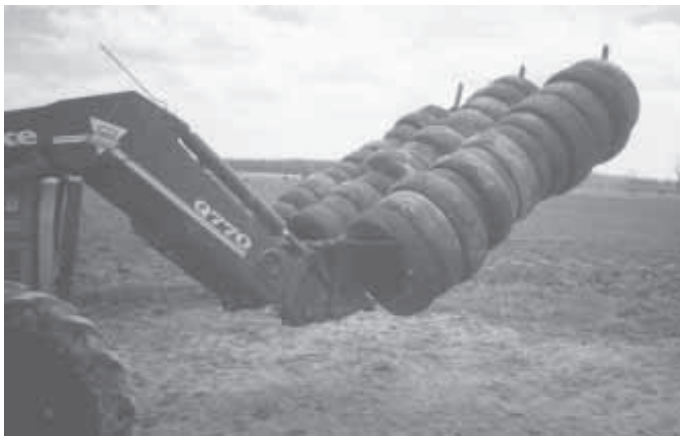
Three-pronged fork fits on a front-end loader and holds 40 to 46 tires at once.
