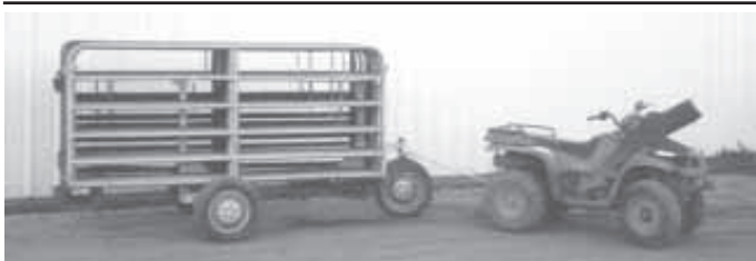
Glen Kesteloot used a new car axle and one front wheel to make this 3-wheeled cart which he uses to carry corral panels.
