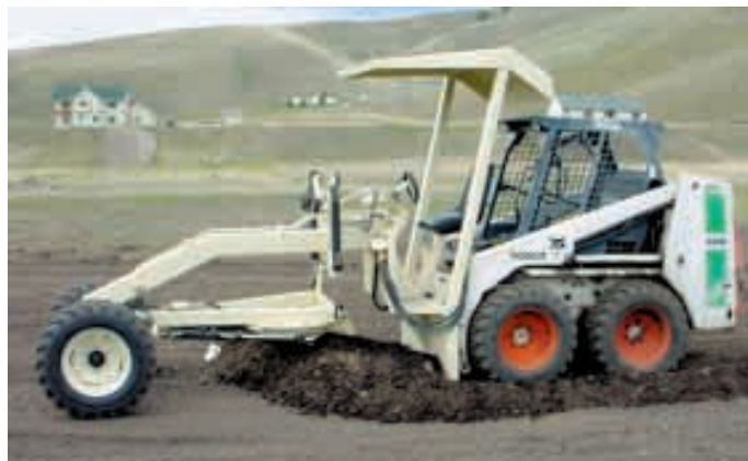
Blade kit quick-taches to skid steer, turning it into a mini road grader. Operator platform is located on grader attachment, providing a clear view of blade at all times.
