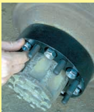
Rear-wheel alignment system puts a spacer between the wheel and hub (left). Auto balancing system (right) also slips onto hub.
