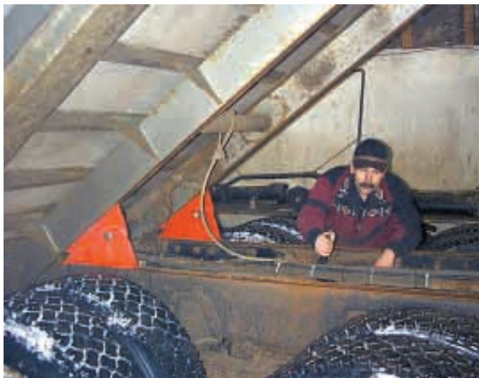
Steel blocks make it safe to work under a raised truck box, without fear of being crushed if hydraulics should fail.
