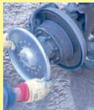
Rear-wheel alignment system puts a spacer between the wheel and hub (left). Auto balancing system (right) also slips onto hub.
