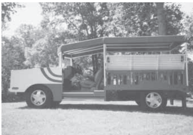
The 20-ft. long vehicle seats two in front and five down each side on 8-ft. long wooden benches. A blue vinyl canopy covers entire passenger seating area.
