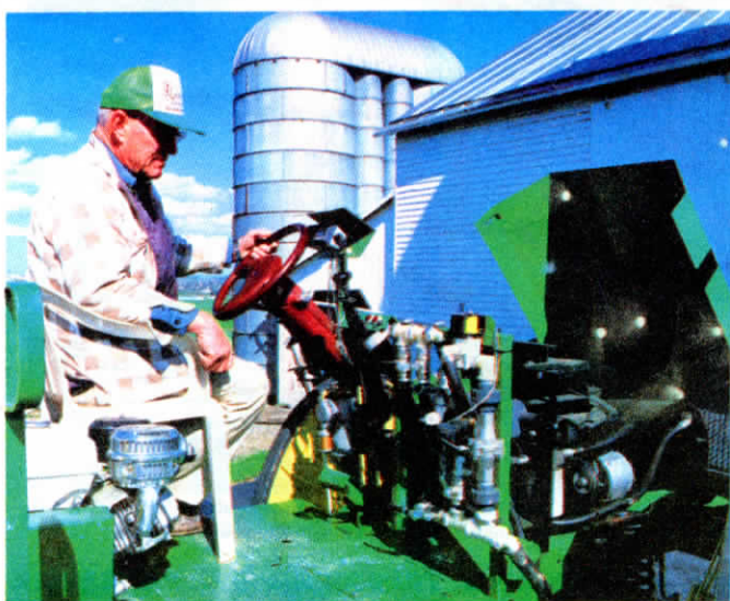
Powered by a lightweight 20-hp. Onan gas engine, all controls are within easy reach of operator. Hydraulic pump and reservoir mount under hood.
