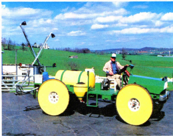
Alger started with the frame from a Ford Ranger pickup. He fitted it with thin steel wheels made by welding steel circles to wheel rims and running reinforcing spokes outward from the rims to the edges of each wheel.
