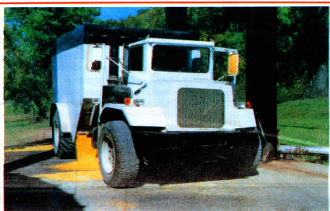
Powered by a lightweight 20-hp. Onan gas engine, all controls are within easy reach of operator. Hydraulic pump and reservoir mount under hood.
