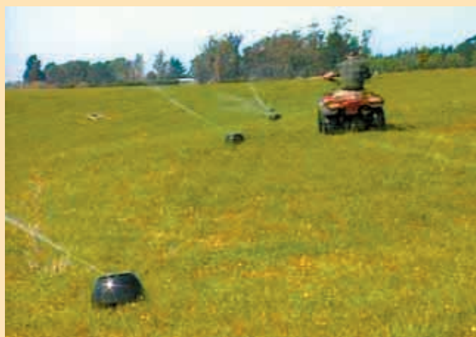
K-Line system consists of a series of tough plastic pods spaced 50 ft. apart and connected by flexible poly pipe. Pods protect sprinklers from livestock.
