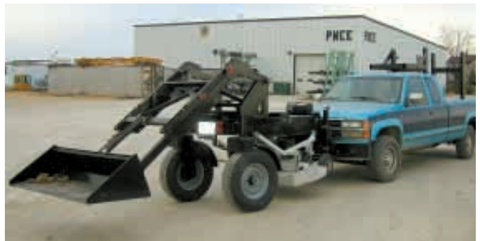
“Carry-All” hooks up to the front of any 4-WD pickup, tractor or skid steer loader. Its frame is equipped with a universal 3-pt. hitch and mounting for a front-end loader.
