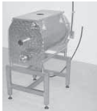
Pladot’s mini pasteurizer, above, is used for pasteurizing milk, juice and egg products. Butter churn, below left, holds 8 gal. and makes 30-lb. batches of butter. Bot- tler, below right, can be used for a variety of products.
