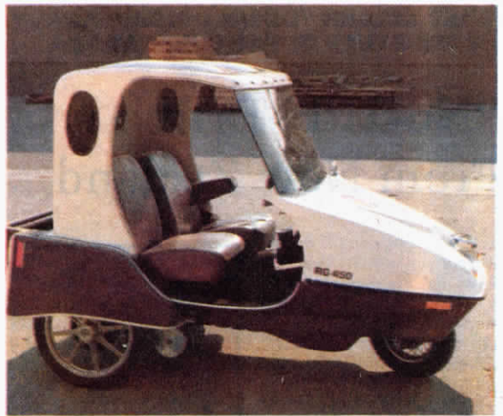
Roadrunner Galaxie travels 30 to 60 miles on each charge of its four 6-volt batteries.
