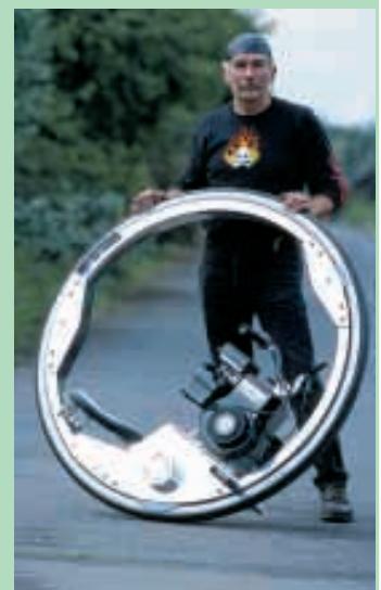
Rig is powered by a 50 hp, water-cooled, 2-cyl. snowmobile engine.
