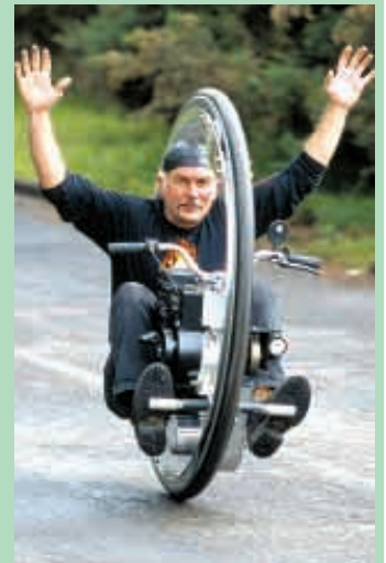
Driver sits astride the engine. Feet ride on a set of pegs mounted on bottom of engine, while a set of pegs atop the engine serves as handlebars.
