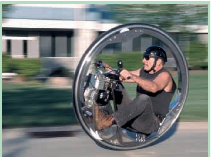
"It's a fun toy to ride," says Kerry McLean about his "Rocket Roadster." A friction drive wheel powers the big outer wheel.
