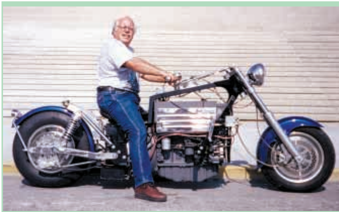
Mick Corse put an industrial 180 cu. in. Deutz air-cooled engine in this home-built motorcycle. Top speed is 108 mph.
