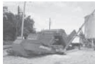
Stationary grain mill is positioned by storage bins. It cleans the crop with a conventional cylinder and sieves.
