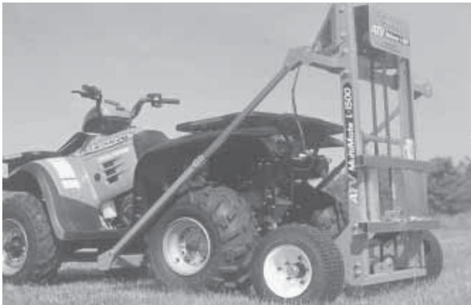
Universal attachment hooks on to nearly any 4-wheel ATV, allowing you to use it as a log skidder, forklift, backhoe, grader, dump bucket, etc.
