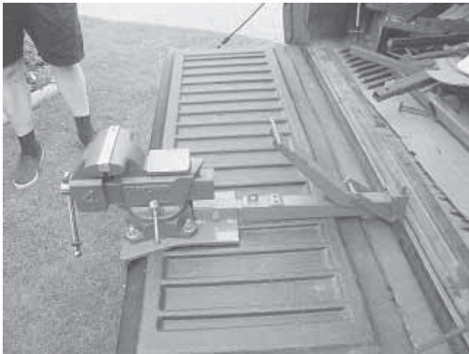
Homemade bracket allows Henderson to quickly attach a vise to the tailgate on his pickup and use it as a workshop in the field.
