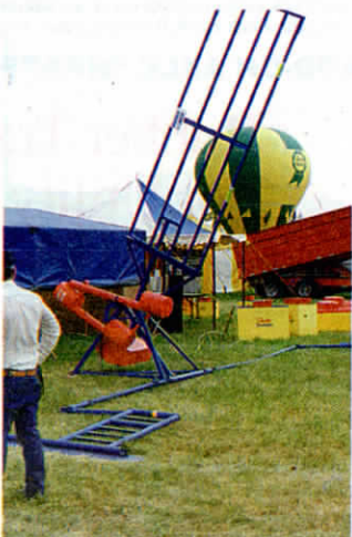
Gate opens up after you drive vehicle onto steel "lift pad".
