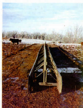
Tow bar fitted with a universal joint mounts on one end of each section of bunk so sections can be ganged together.
