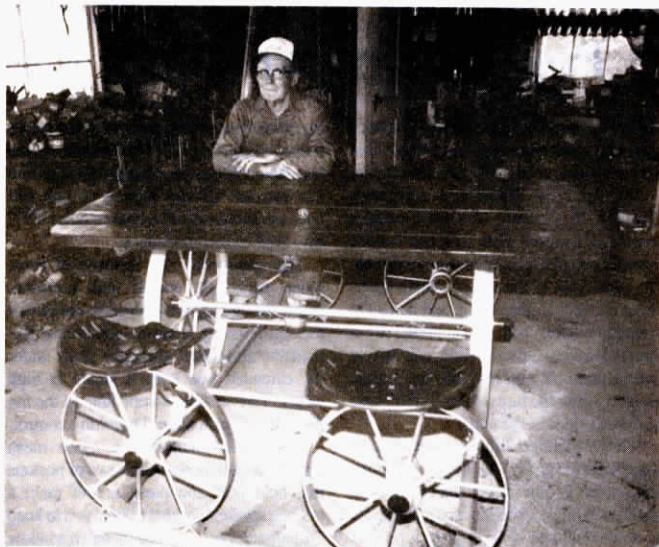
Amos Miller welded four horse-drawn rake and mower seats to the tops of four wheels which he salvaged from a 1920's era horse-powered hay baler.
