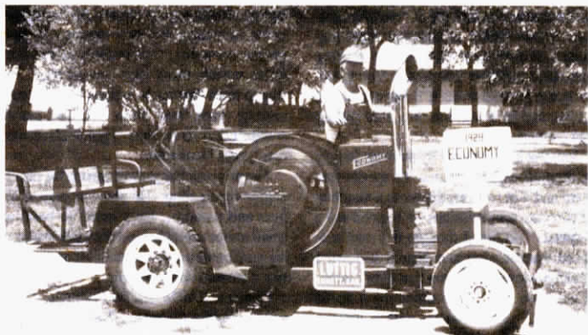
Luttig hooked up a 1928 Sears "one lunger" engine to a 3-speed transmission.
