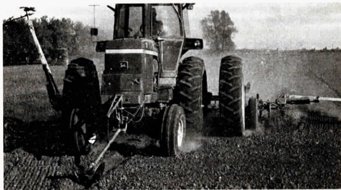
TAG System's sensor arm rides in furrow made by power marker and completely steers tractor going down the row.
