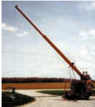
Manure pump hangs from cable at end of boom.
