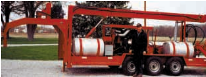
Specially designed tri-axle gooseneck trailer hauls pump, engine, and 200-gal. fuel tank.
