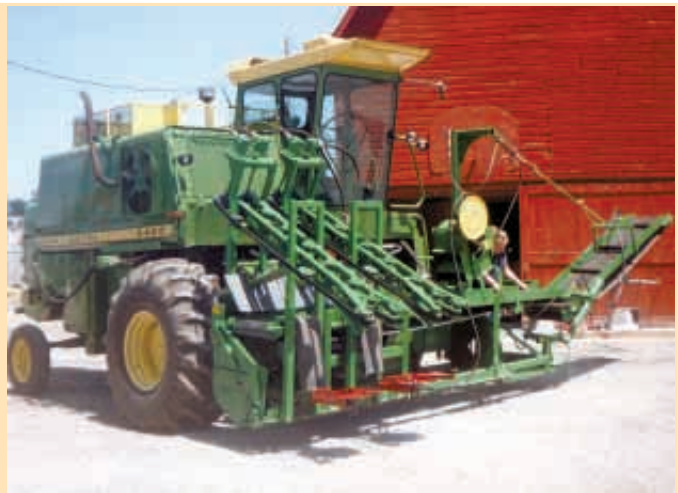
Home-made picker mounts in place of header on conventional combine. It uses belts to grab corn stalks and knives to cut them 1 ft. above ground. Rollers strip ears off and deposit them in a bulk wagon.
