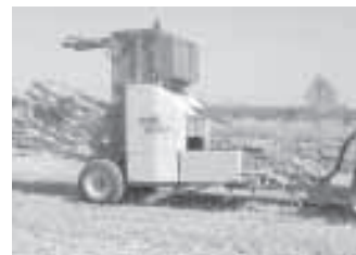
Buncher picks small bales up off field, packs 14 together, and ties them up into one bundle which it drops back onto field.
