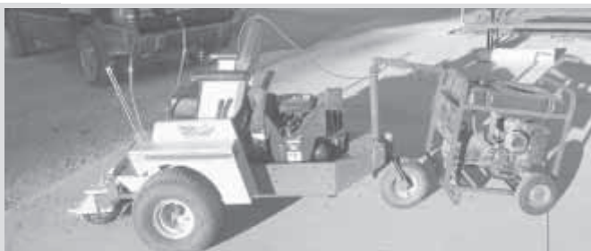
Rich DeVries mounted two DC motor coils on front of his Grasshopper lawn mower in place of the deck. Magnets are powered by a generator pulled behind mower.
