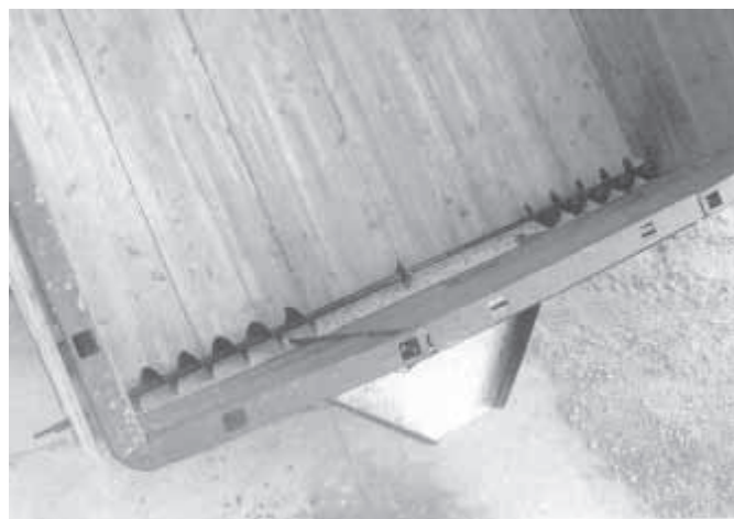
Hand-cranked clean-out auger eliminates need to climb inside truck box.
