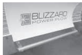
Pipe on bottom of snow blade is used to skim snow off grass on Keith Myer's private airfield.
